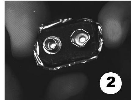
2. After you pry back the rim of the battery casing, the exposed connector plate can be removed.
