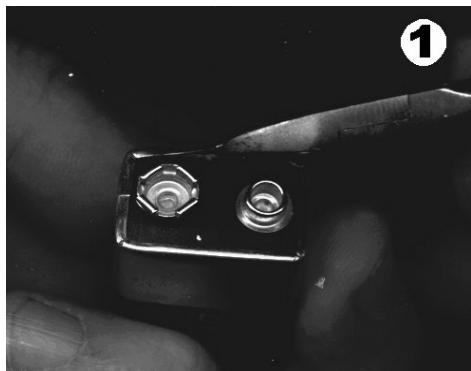
1. Once you know a battery has no life in it. Pry the metal casing off from around the top with your choice of pliers. This is a dead Duracell but the casing is generally identical in other batteries.
